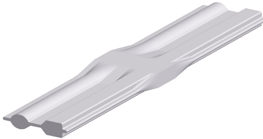
Computer model of Cornell ERL vacuum chamber transition
