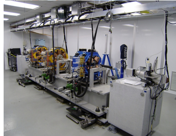
Environmental Room ( \Delta T < 0.1\text{ C} ) for 30\text{ }\mu\text{m} Precision Alignment
