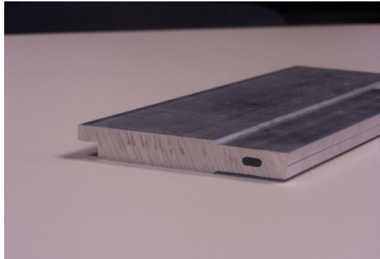
Section of extrusion
