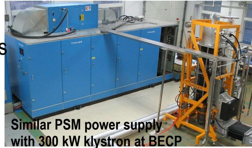
Similar PSM power supply with 300 kW klystron at BECP
