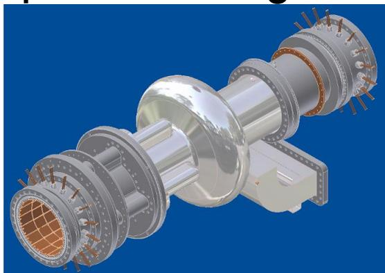
Waveguide aperture coupling with capacitive tongue to cavity beam pipe
