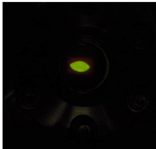
Figure 2: Digital photograph of a 1 \mu s beam pulse taken during an operation at a repetition rate of 1 Hz.
