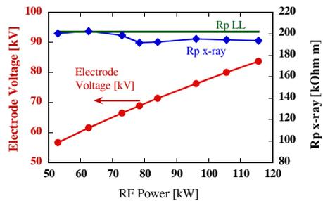
Figure 4: X-ray endpoint calibration of the inter electrode voltages and verification of the nominal shunt impedance.
