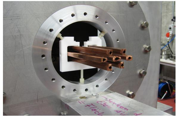
Figure 5: The new matching section with the nonconducting stem.
