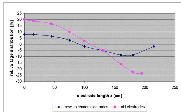
Figure 8: Longitudinal voltage distribution in the RFQ.
