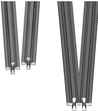
Figure 4: The old (left) and new (right) end of the matching section.
