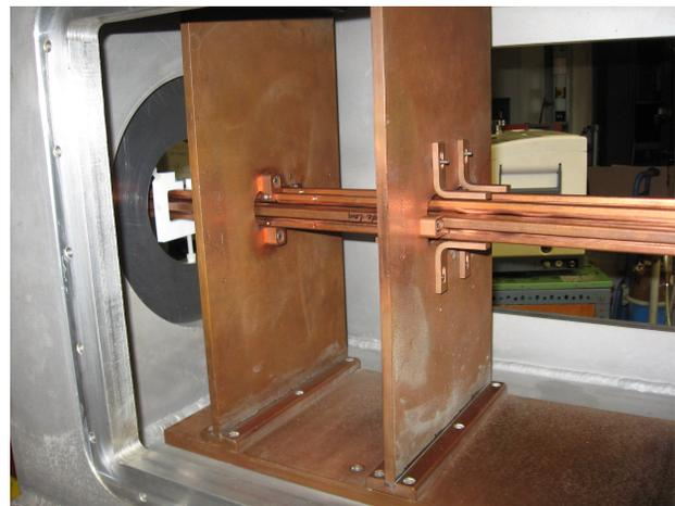
Figure 7: Small tuning angles as additional capacity for a better voltage symmetry.
