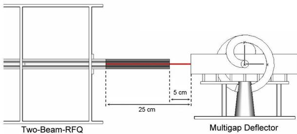
Figure 3: Old drift (without) and new drift (with gray part) between RFQ and deflector.
