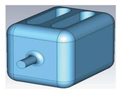
Figure 1: TEM-type superconducting cavity Ref. [12].
