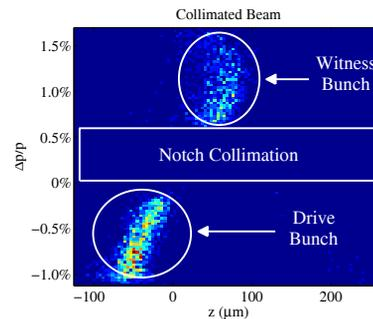
Figure 1: Longitudinal phase space at the IP, 10 mm  $R_{56}$ , with momentum tail and notch collimation. Drive bunch ( $z$  std. dev.  $23 \mu\text{m}$ ) is at left with lower energy, the witness bunch ( $z$  std. dev.  $18 \mu\text{m}$ ) at right with higher energy. Bunch separation is  $120 \mu\text{m}$ , with a charge ratio of 1.6.
