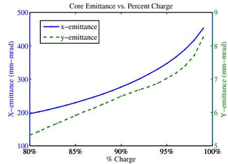
Figure 3: The large growth at higher percentage indicates inclusion of halo particles. 95% beam charge represents the core emittance without this large growth.
