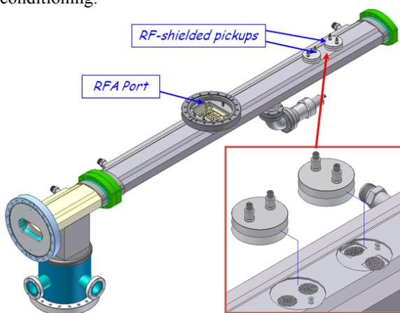
Figure 6. This design of aluminium chamber is used in the short experimental sections at Q15W and Q15E in CESR.
