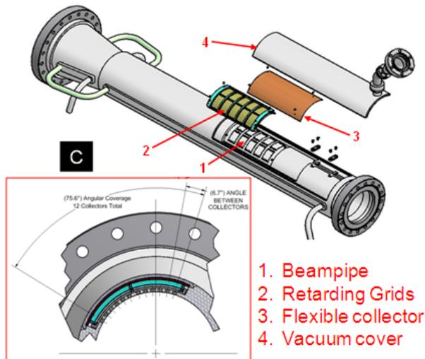
Figure 5: Implementation of thin RFA in a quadrupole vacuum chamber
