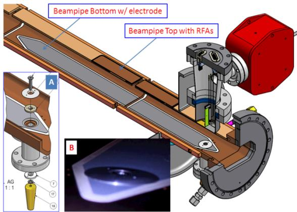
Figure 2: RFA SCW beampipe with a clearing electrode. The electrode was deposited onto the bottom half of the beampipe via thermal-spray technique. Insert A illustrates structure of low-profile electric contact, and insert B is an image of the contact button taken during post operation inspection in January 2011.
