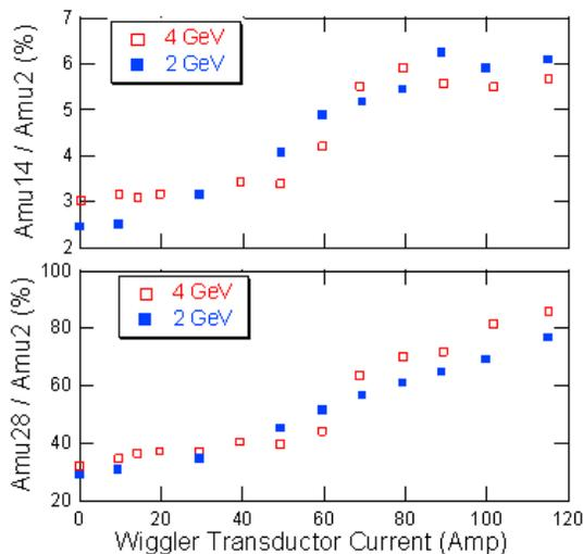
Figure 3: Increased desorption of N<sub>2</sub> from TiN coated surfaces with increasing magnetic field in the SCWs. The measurements were taken with a 35 mA positron beam at beam energies of 2 and 4 GeV.
