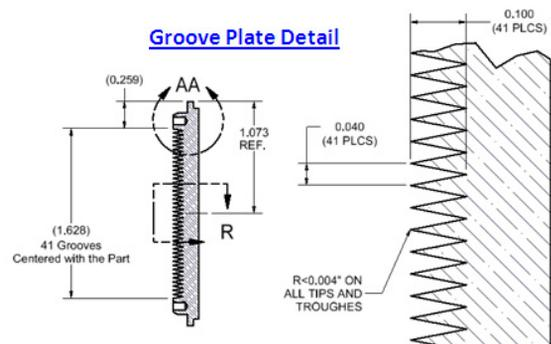
Figure 1: Detail of grooved plate welded into SCW beampipe. The plate is copper with 41, 1mm spaced triangular grooves.
