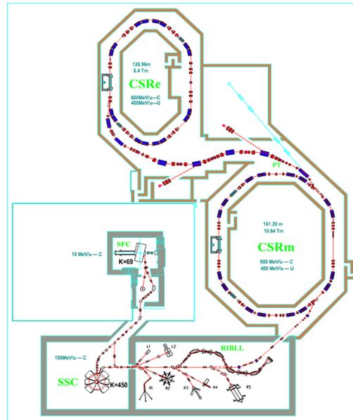
Figure 1: Overall layout of HIRFL-CSR.
