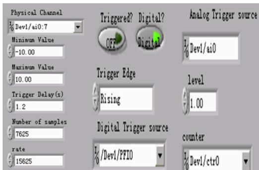
Figure 3: Settings interface of ADC card.
