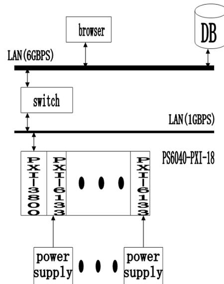
Figure 2: Whole structure of hardware.
