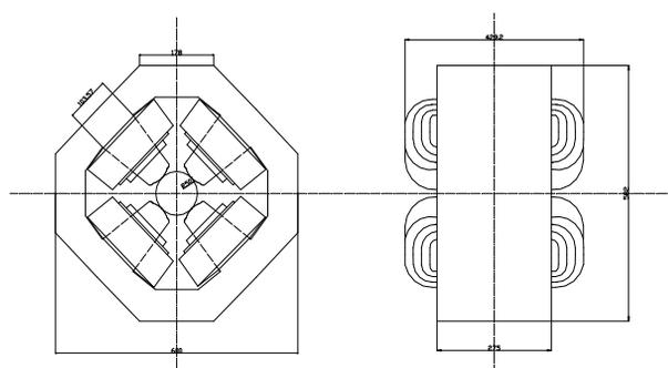
Figure 2: End view and overhead view of the quadrupole magnet.
