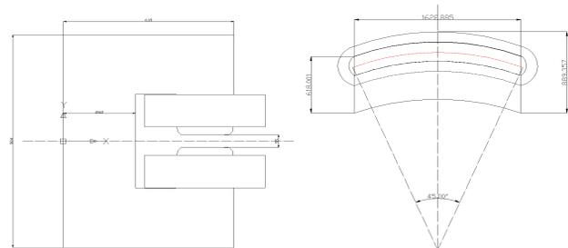
Figure 1: End view and overhead view of the dipole magnet.
