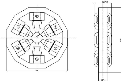
Figure 3: End view and overhead view of the sextupole magnet.
