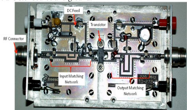
Figure 8: Prototype driver amplifier.
