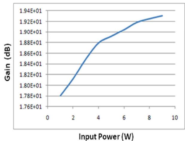
Figure 12: Measured gain of driver amplifier.
