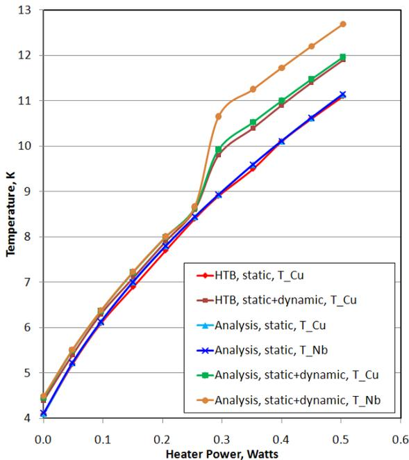
Figure 7: Temperatures from analysis and HTB tests.
