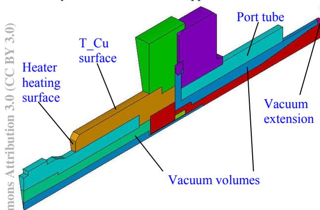
Figure 3: A wedge model of HOM feedthrough.
