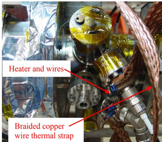
Figure 2: HOM coaxial couplers in HTB cryomodule.
