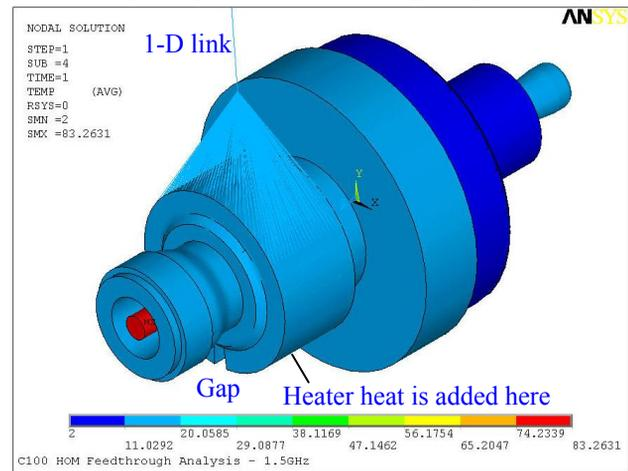
Figure 8: Temperature in a full model when the heater power is 503 mW.
