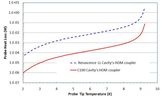
Figure 4: Niobium probe tip heat vs. Temperature at  $E_{acc} = 20\text{MV/m}$  by 3D RF code (HFSS or Omega3P).
