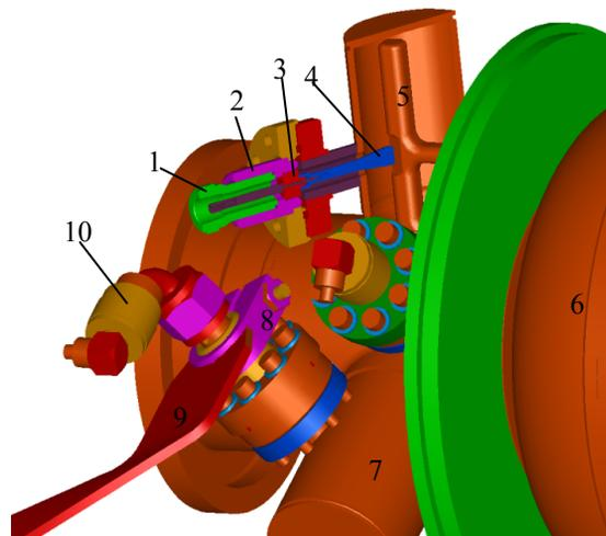
Figure 1: HOM coaxial couplers on JLAB 12 GeV upgrade cryomodule cavity end group (some components are abridged for clarity): 1. Type N connector; 2. Cu sleeve; 3. Sapphire ring; 4. Nb probe; 5. Nb hook; 6. Nb cavity; 7. HOM can; 8. Cu bracket; 9. Cu thermal strap; 10. Elbow adapter.
