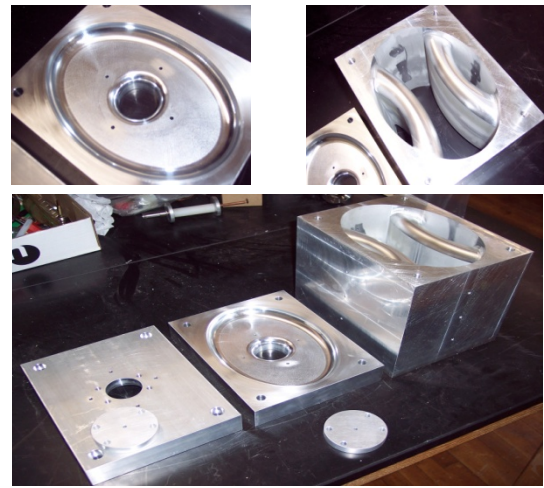
Figure 4: 800 MHz elliptical shaped cavity prototype.
