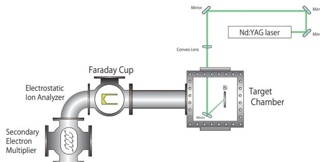
Figure 1: LIS experimental sketch for low charge Bismuth ions. The total current distribution was measured by Faraday Cup (FC). Electrostatic Ion Analyzer (EIA) with Secondary Electron Multiplier (SEM) analyzes the charge state distribution.
