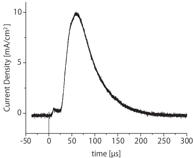
Figure 2: Total current density of Bismuth ions was measured by FC.
