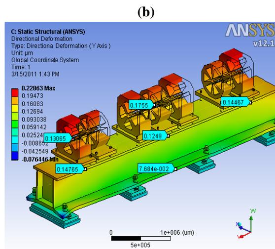
Figure 4: (a) Measured time-temperature girder response,  $\Delta T_{Girder} = (1/10)\Delta T_{Air}$ , (b) FEA girder deflection (deflection < 25 nm for  $\Delta T_{Girder} \sim 0.01$  °C).
