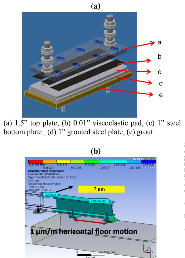
Figure 8: (a) Girder mounting base design incorporating the viscoelastic material, (b) FEA vertical deflection of girder with the viscoelastic pad.
