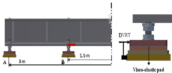
Figure 9: Thermal-testing scheme for the girder with viscoelastic pads.
