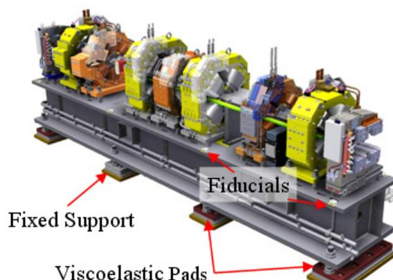
Figure 1: NSLS-II girder support system design.
