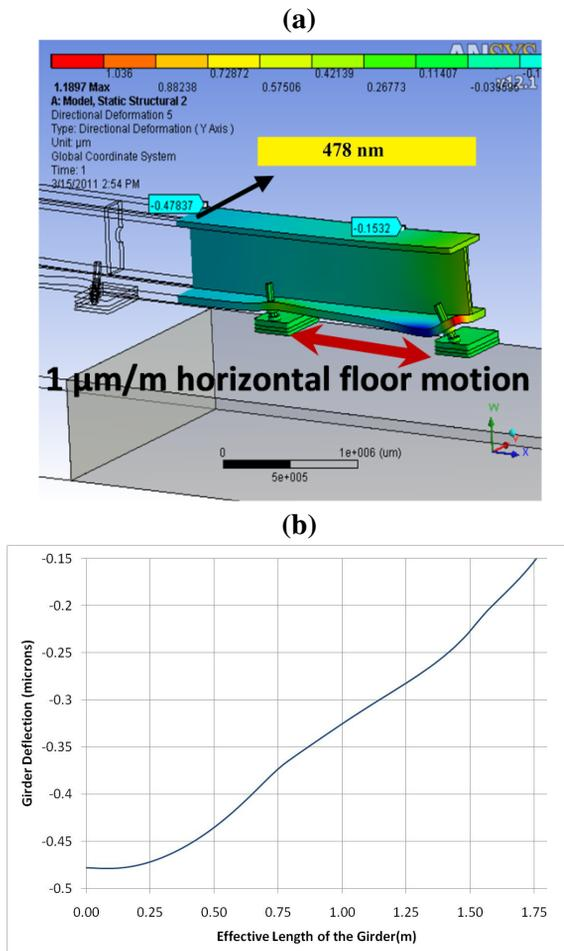
Figure 7: (a) FEA results - girder deflection due to diurnal floor expansion, (b) Girder deflection over the effective girder length.
