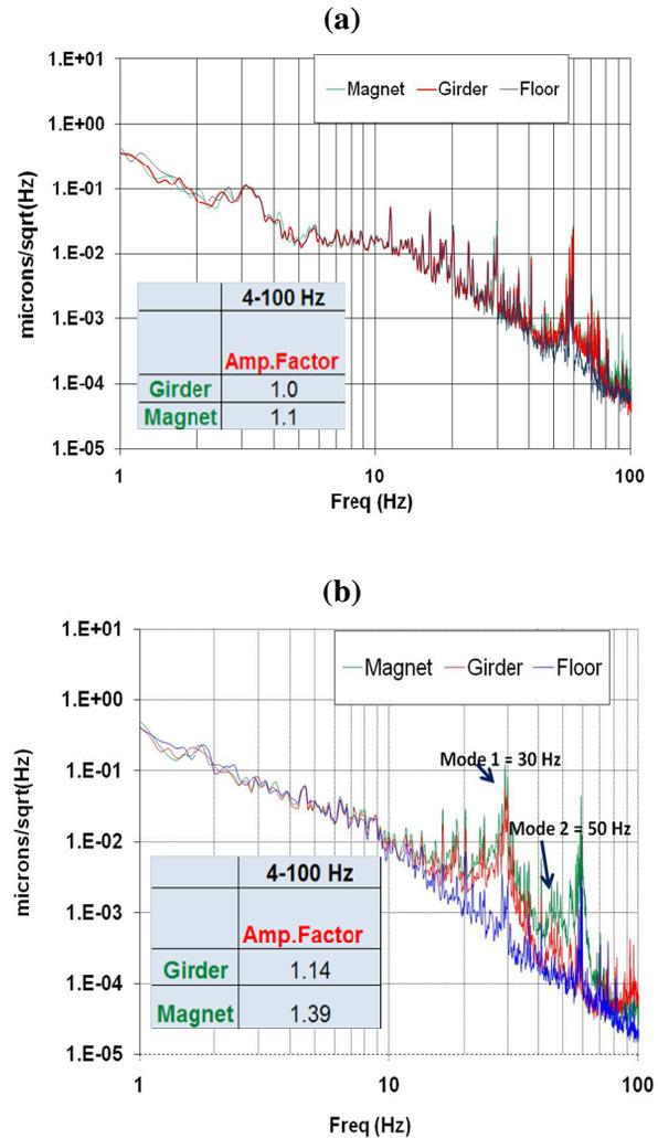
Figure 3: Random vibration tests: (a) Vertical  $\sqrt{\text{PSD}}$ , (b) Horizontal  $\sqrt{\text{PSD}}$ .
