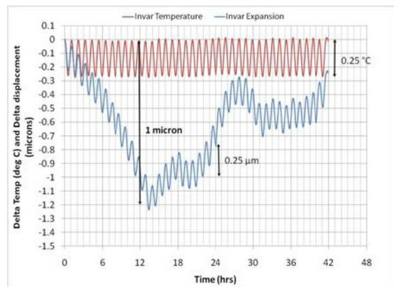
Figure 6: Displacement and temperature variation of an invar rod in a thermally stable environmental room.
