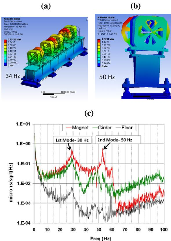
Figure 2: (a) 1<sup>st</sup> rocking mode of vibration, ~30 Hz, (b) - 2<sup>nd</sup> twist mode of vibration, ~50 Hz, (c) Vibration response of a girder-magnet assembly subjected to impact loading.
