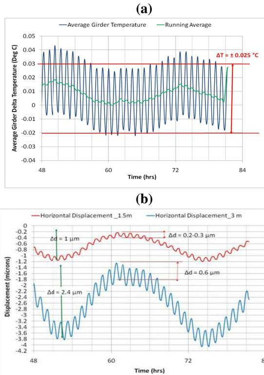
Figure 10: (a) Girder temperature variation, (b) Relative horizontal displacement between the girder and the floor.
