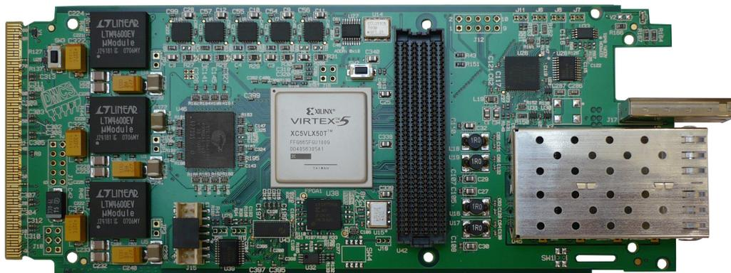
Figure 2. Assembled AMC Univerlas Module
