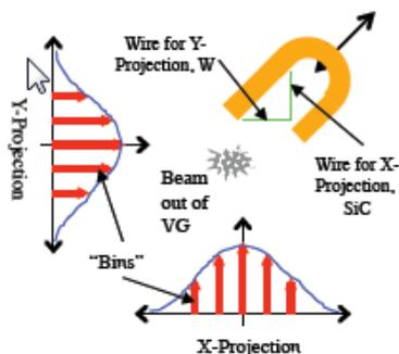
Figure 1: wire scanner basics diagram.
