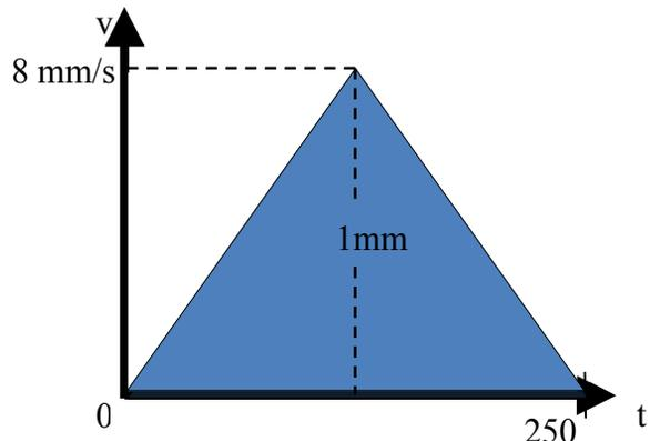
Figure 2: Velocity profile for the wire scanner.
