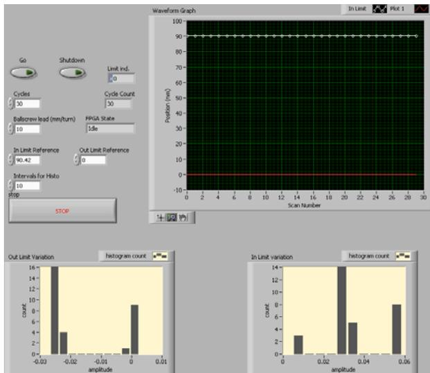
Figure 5: Limit switches repeatability test.
