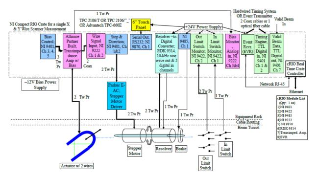
Figure 1: LANSCE-R Wire-Scanner System Block Diagram.
