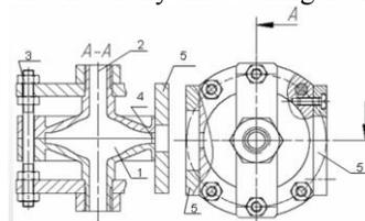
Figure 3: Drawing of the test cavity with a flexible wall: 1 – cavity body; 2 – simulated beam tunnel; 3 – tuning screw, 4 – coupling holes; 5 – waveguide flanges.
