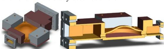
Figure 2: Bimodal cavity in a clamped structure with demountable bottom surface.
