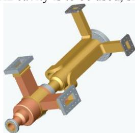
Figure 6: RF structure for second harmonic power source.
