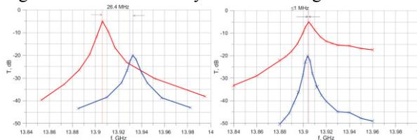
Figure 4: Measured transmission vs frequency: (a) before cavity deformation, (b) after cavity deformation. Red curve corresponds to 14 GHz mode, blue curve corresponds to 7 GHz mode, whose transmission is plotted as function of  $2 \times f$ .
