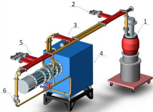
Figure 5: Layout of dual-frequency RF source, shown feeding a bimodal test cavity. 1 – S-band klystron; 2 – variable power splitter; 3 – 3-dB hybrid splitter; 4 – 250-kV electron gun tank; 5 – variable power splitter and phase shifter; 6 - bimodal test cavity. Gray structure attached to gun tank is the magnetic circuit, within which the two-cavity source is positioned.
