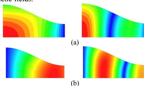
Figure 1: (a) The electric field map and (b) the magnetic field map for 2.856 GHz  $TM_{01}$  and 5.712 GHz  $TM_{02}$  modes.
