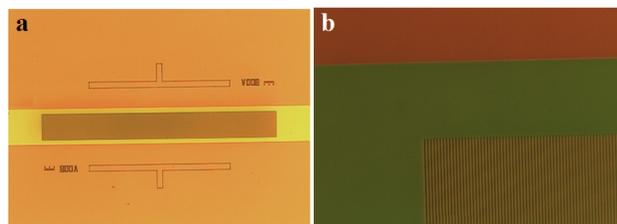
Figure 6: Bottom layer of the accelerator structure with nitride spacer layer and vacuum channel in place.
