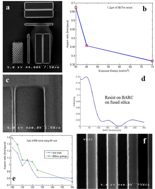
Figure 3: Lithography optimization: a) Test pattern, b) exposure trend with standard resists, c) sample over-exposed pattern, d) Reflectivity improvement using AR coat, e) exposure trend with AR coat applied, f) sample exposed grating pattern using AR coat.
