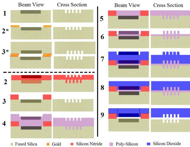
Figure 2: Fabrication Process for the dual layer grating structure. Steps described in the text.
