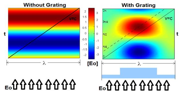
Figure 1: Grating structure principle of Operation: each grating pillar provides a  $\pi$  phase delay such that at the right phase the e-beam experiences net acceleration.
