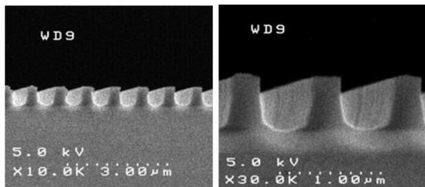
Figure 4: Cross-section of an etched 800nm grating.
