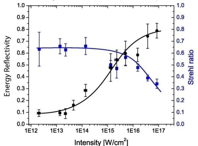
Figure 3: Energy reflectivity (black circles) and Strehl ratio (blue squares) as a function of the laser intensity. The solid lines are used to guide the eyes.
