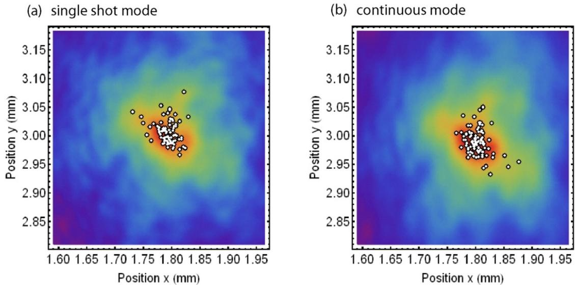
Figure 4: Beam pointing measurement for (a) single shot mode and (b) continuous mode. The white dots represent the centroid of the beam for each individual measurement. The background is the sum of all measurements.
