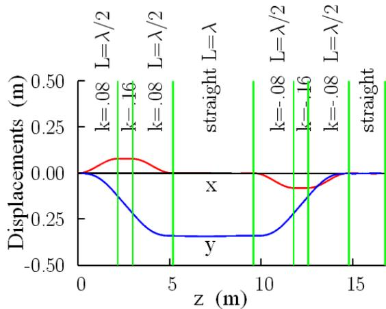
Figure 5: Central track in the 400 MeV example.  $x, y, z$  are transport coordinates.
