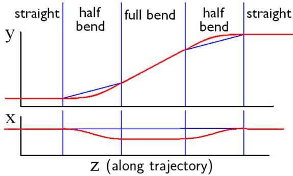
Figure 3: Norem's method to match entry and exit of bent solenoid.  $x, y, z$  are transport coordinates.
