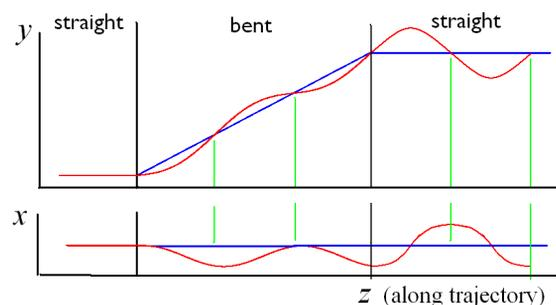
Figure 2: Uncorrected entry and exit from a bent solenoid.  $x, y, z$  are transport coordinates.
