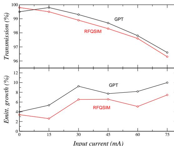
Figure 4: Successful particle transmission (top) and emittance growth (bottom) as a function of the input current, calculated by RFQSIM and GPT.
