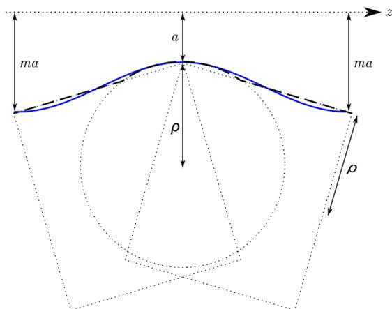
Figure 3: Representation of the vane profile approximated by spheres and inclined cylinders. The spheres are created with radius  $\rho$  and centered at  $a + \rho$ , and the inclination of the cylinders is calculated so that their upper edges join consecutive minima and maxima vane apertures.
