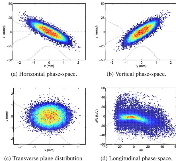
Figure 2: Particle density plots at the output of the RFQ.
