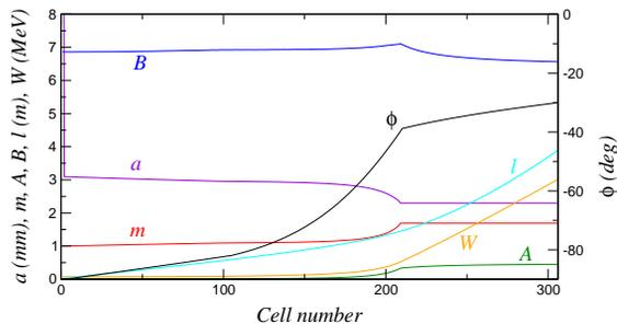
Figure 1: Evolution of several RFQ parameters as a function of the cell number.
