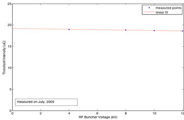
Figure 7: e-p instability threshold versus RF 1<sup>st</sup> harmonic amplitude.
