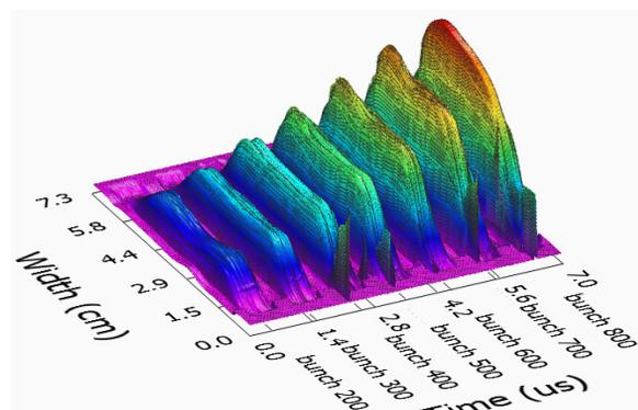
Figure 1: Evolution of a  $1 \times 10^{14}$  ppp beam during beam accumulation. Beam is shown for turns 200, 300, 400, 500, 600, 700, and 800, with a 25ns time resolution within a turn.
