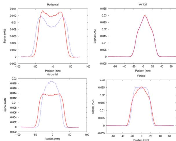
Figure 3: Horizontal and vertical profiles (top) for two different horizontal injection kicker settings. The corresponding profiles when the tune split was 0.1 (top) and 0.03 (bottom).
