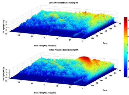
Figure 11: Data for a Feb 2011 production beam, showing the vertical plane frequency space during accumulation for beam with (top) and without (bottom) the transverse feed back system on.
