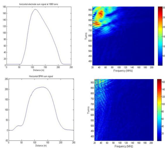
Figure 8: The bunch shape and corresponding frequency spectrum for two beams with a 35 degree difference in the 2<sup>nd</sup> harmonic RF phase.
