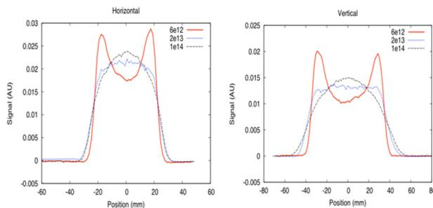
Figure 2: Horizontal and vertical profiles of the beam after extraction from the ring for three different beam intensities but the same painting scheme.
