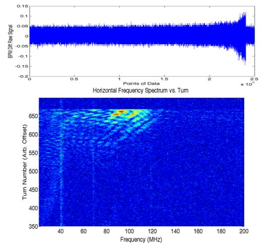
Figure 9: Raw BPM data (top) and the processed data for frequency versus turn.
