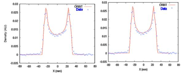
Figure 12: Benchmark of horizontal beam profiles for a painted beam with 2.2e12 ppp (left) and 7.5e13 ppp (right). The red line is the simulation, and the blue dots are the measurement.
