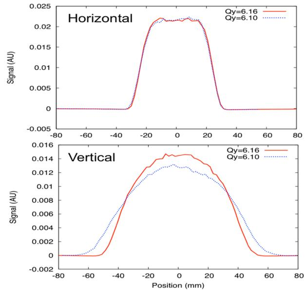
Figure 6: RTBT wirescanner profiles, for a  $1.2e14$  ppp beam with vertical tunes  $Q_y=6.16$ , and  $Q_y=6.10$ . The horizontal tune was fixed at  $Q_x=6.20$ . top.
