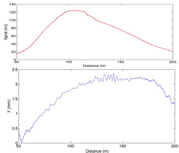
Figure 10: Bunch intensity and position for a portion of a single turn of beam near the end of the accumulation cycle for the beam shown in Fig. 9.
