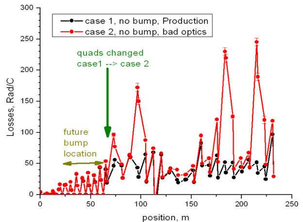
Figure 9: The SCL beam loss monitor signals for two optics set-ups without the closed trajectory bump.
