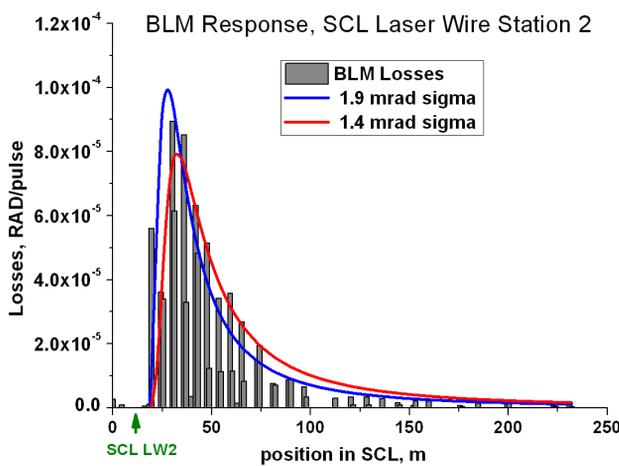
Figure 3: Loss distribution in the SCL after stripping of the H<sup>-</sup> beam by the laser beam. The bars are BLM responses, blue and red curves are the simulated distributions for different Gaussian angular distributions of the ion beam.
