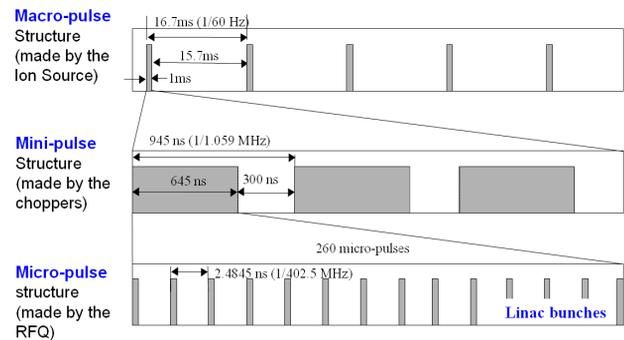
Figure 4: The time structure of the SNS linac beam.
