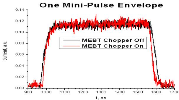
Figure 5: The envelope of one SNS linac mini-pulse and the effect of MEBT chopping.
