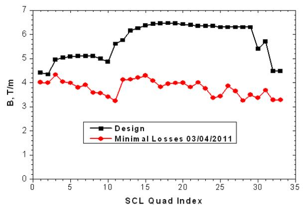
Figure 7: Quadrupole gradients for design and production.
