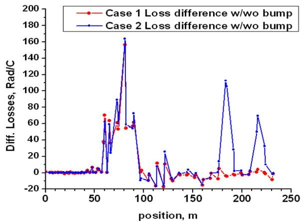
Figure 10: The SCL beam loss change after the closed trajectory bump was created.
