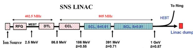
Figure 1: The structure of the SNS linac.
