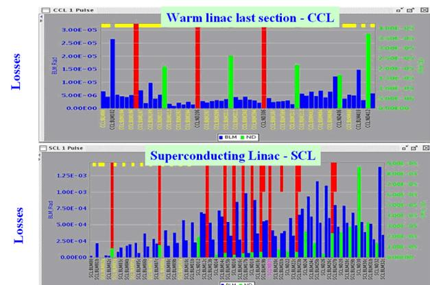
Figure 2: The production losses in the CCL and SCL.
