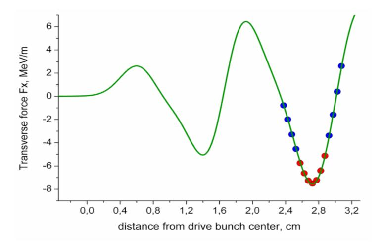
Portrait of test particles at initial transverse locations in the witness channel at input to structure.
