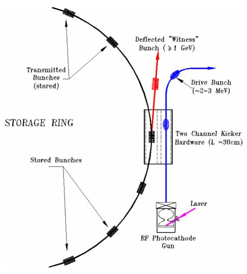
A rectangular two-beam dielectric wakefield accelerator (DWFA) is under study in a collaboration between Omega-P, Yale, Columbia, and ANL. Due to asymmetry, this stucture will deflect a test bunch moving in the narrow channel, due to wake fields set up by drive bunches in the broad channel.
