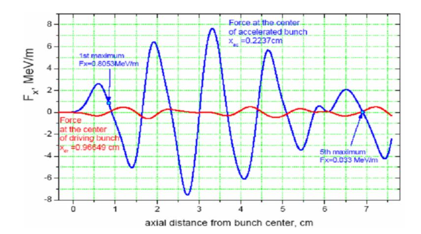
Calculated x-component of transverse deflection of nine 1-GeV test particles in a 30-cm long two-channel rectangular test module
