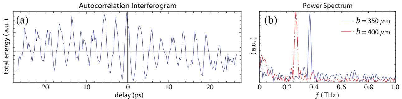
Figure 4: (a) Typical measured autocorrelation interferogram of radiation from  $b = 350 \mu\text{m}$  tube. (b) Measured power spectra, calculated by discrete Fourier transform, of radiation from  $b = 350$  and  $400 \mu\text{m}$  tubes.
