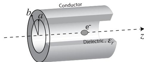
Figure 1: Cutaway diagram of a cylindrical dielectric-lined waveguide structure.
