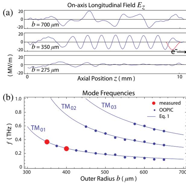
Figure 2: (a) OOPIC simulation of longitudinal wakefield  $E_z$  on tube axis vs. position along tube, for increasing  $b$  with fixed  $a$  and  $\sigma_z$ . (b) Scaling of mode frequencies with  $b$ , for constant  $a = 250 \mu\text{m}$  and  $\sigma_z = 200 \mu\text{m}$ .
