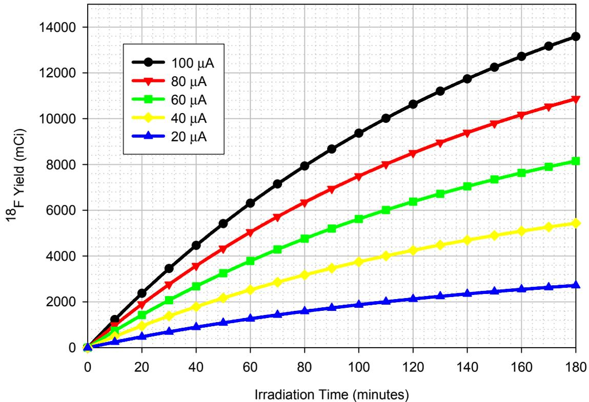
Figure 1: Production yield curves for the Bruce Technologies Inc. CF-1000 Target.
