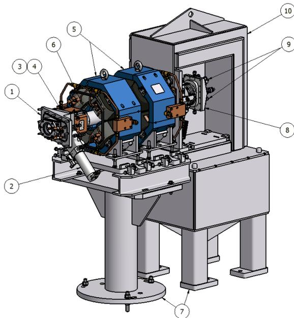
Figure 2: Compact 1.1 metre beamline designed by D-Pace for THC-14 PET Cyclotron [2,4]. (1) Graphite Exit Port Baffle with Beam Current Readback, (2) Gate Valve, (3) XY Steering Magnet, (4) Bellows, (5) Quadrupole Doublet, (6) Aluminium Beampipe, (7) Supports, (8) TRIUMF Target Selector, (9) CF-1000 Target, (10) Lead/Polyethylene Shielding.
