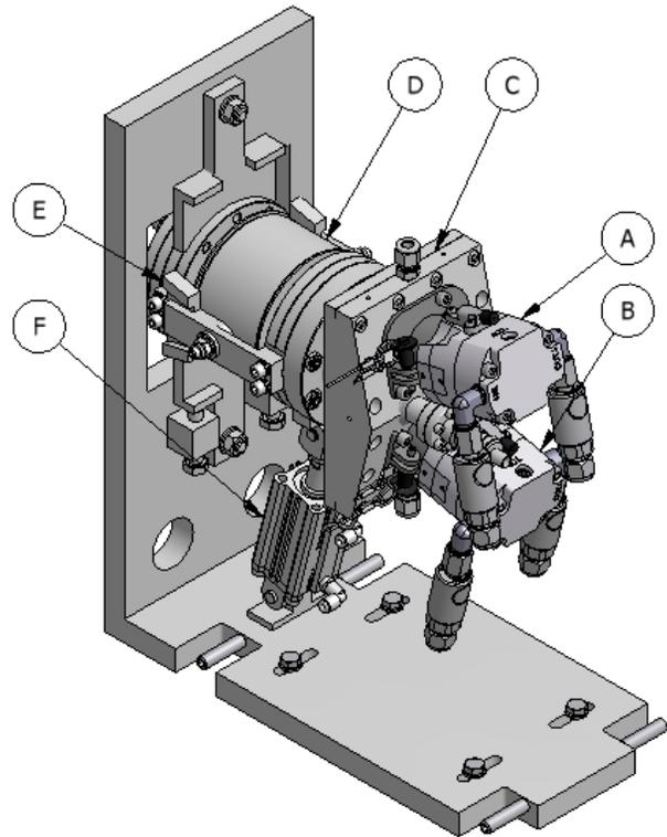
Figure 3: TRIUMF Licensed target Selector with (A, B) Bruce Tech CF-1000 water targets, (C) Housing with Graphite water-cooled baffle and 4-jaw collimators with beam current readbacks, (D) Bellows, (E) Angle Bracket Alignment Structures, (F) Piston.
