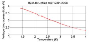
Figure 7: Temperature dependence of the voltage drop across diode 1N4148 when 5 V was applied at  $V_a$  in Fig. 6.
