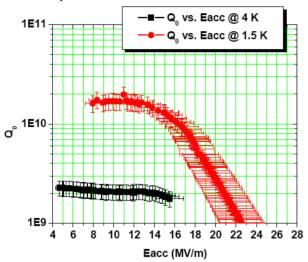
Figure 5: Q<sub>0</sub>-E<sub>acc</sub> curve of the 805 MHz single cell cavity.
