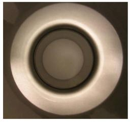
Figure 3: The cavity inside surface after BCP. This side was facing upward during BCP.
