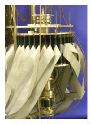
Figure 4: The 805 MHz single-cell cavity surrounded by temperature mapping boards.
