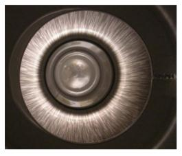
Figure 2: The cavity inside surface after BCP. This side was facing downward during BCP. The surface looked similar to Figure 1.
