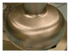
Figure 1: Outside surface after BCP of 150  $\mu m$ . This side was facing downward when BCP was done. Traces of bubbles are clearly seen. The surface facing upward was smooth.
