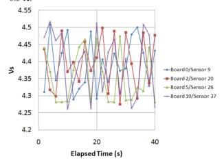
Figure 8: T-map noise level of 4 sensors measured at 4 K. The horizontal axis corresponds to the data number. The data taking time per sector is 2 s.
