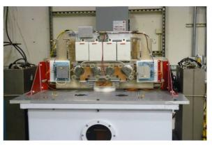
Figure 7: Single-phase H-bridge test stand
