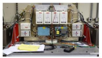
Figure 2: Existing H-bridge switch plate on SLAC test stand.
