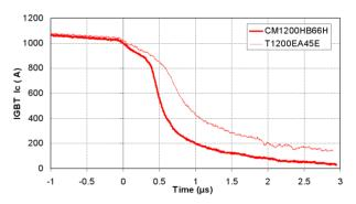
Figure 6: Comparison of the turn-off Ic waveforms for two different IGBTs.
