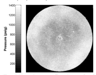
Figure 4: Measured pressure profile on the top surface of press-pack IGBT.
