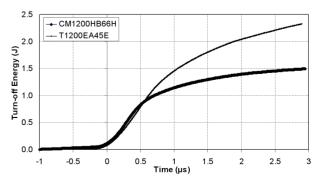
Figure 7: Comparison of the turn-off energy waveforms
