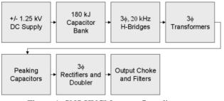
Figure 1: SNS HVCM power flow diagram.
