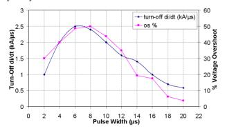
Figure 5: Measured turn-off di/dt for the press-pack IGBT at a capacitor charge of +/- 400V. The di/dt magnitude correlates with the percentage voltage overshoot (OS).
