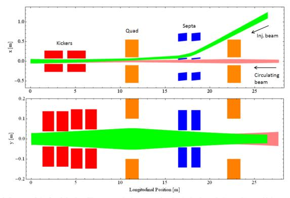
Figure 2: Layout of the fast injection. The top graph shows the view in the horizontal plane with two kicker tanks, the lower graph with four kicker tanks in the vertical plane, where the aperture available for the beams is drawn instead of the magnet aperture. The beam sizes plotted correspond to the required aperture  $A_{x,y}$ .
