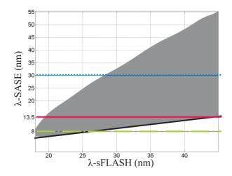
Figure 2: Assuming a seed pulse energy of 1 nJ, the gray area represents working points where saturation of the FEL is expected for a given set of FLASH SASE-wavelengths and sFLASH-wavelength.
