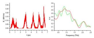
Figure 4: Electric field component *y* for the five pulses bunch (left) and comparison between the field FFT, in red, and the beam form factor, in green (right).
