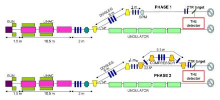
Figure 1: Cartoon of the SPARC photoinjector with a THz radiation station in phase 1 (upper) and 2 (lower). A magnetic compressor is foreseen in the second phase only. Bending and quadrupole magnets are marked by yellow wedges and blue lenses, respectively.
