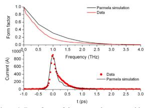
Figure 6: Form factor of the measured compressed beam compared to the simulated one (upper) and corresponding longitudinal beam distribution (lower).
