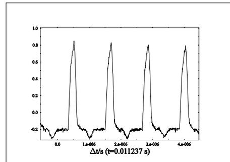
Figure 9: Beam signal after the 90° bunch-rotation.
