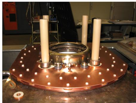
Figure 5: The modified tube socket equipped with fifty 5 nF barrel style capacitors
