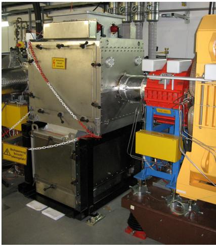
Figure 6: The cavity and power amplifier already installed in the SIS18-tunnel
