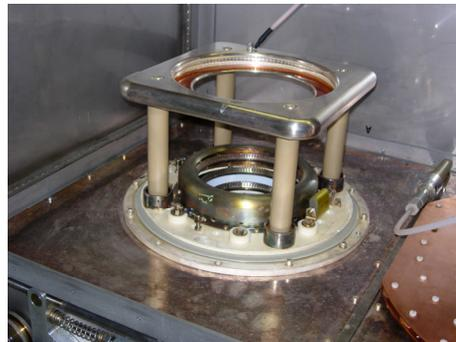
Figure 4: The original tube socket for the RS 2054 SK tetrode with the film shunt capacitor
