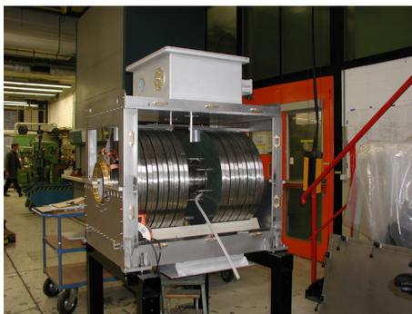
Figure 3: The bunch compressor cavity loaded by 20 MA-ring-cores (VitroVAC 6030F). The box on top of the cavity contains the adjustable gap capacitors to tune the cavity.
