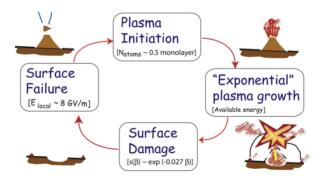
Figure 1: The overall picture of the breakdown cycle.
