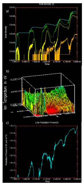
Figure 6: Examples of OOPIC Pro output showing, a) Plasma evolution in the first 7 ns (colors as in Fig. 5),
