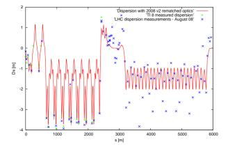
Figure 2: Nominal horizontal dispersion (red line) and measured dispersion values (crosses) from the start of TI 8 to the right of IP7 in the LHC.
