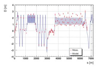
Figure 1: Nominal horizontal dispersion (blue line) and measured dispersion values (red triangles) from the start of TI 2 to the left of IP3 in the LHC.
