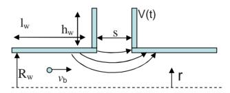
Figure 2: Schematic of the acceleration gap of the induction bunching module. Arrows indicate the direction of the electric field; the dotted line shows the axis of symmetry.
