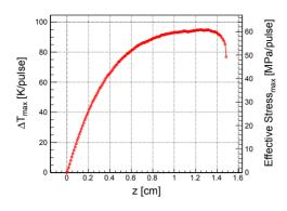
Figure 6: Temperature profile and stress induced by the beam for one pulse in the rotating target for an undulator length of 100.6 m.
