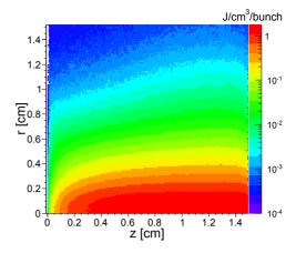
Figure 4: Energy density from a FLUKA simulation of the initial energy deposition into a 15 mm thick Ti-6%Al-4%V target by one bunch of the undulator radiation for  $K=0.92,\,\lambda_0=11.5$  mm and  $d_{\rm UT}=500$  m.
