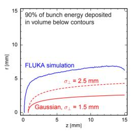
Figure 5: Contour of the energy density under which 90% of the bunch energy is deposited for the FLUKA simulation, Fig. 4, (blue) and Gaussian distributions (red) with radial dimension  $\sigma_{\perp}$ .
