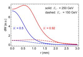
Figure 2: Undulator radiation at target surface for  $E_{e^-}=250~{\rm GeV}$  (solid) and  $E_{e^-}=150~{\rm GeV}$  (dashed) with  $d_{\rm UT}=500~{\rm m},~K=0.92$  (red) and K=0.5 (blue) in the normalization  $dW(K=0.92,E_{e^-}=150~{\rm GeV},\theta\to0)\equiv1$ .
