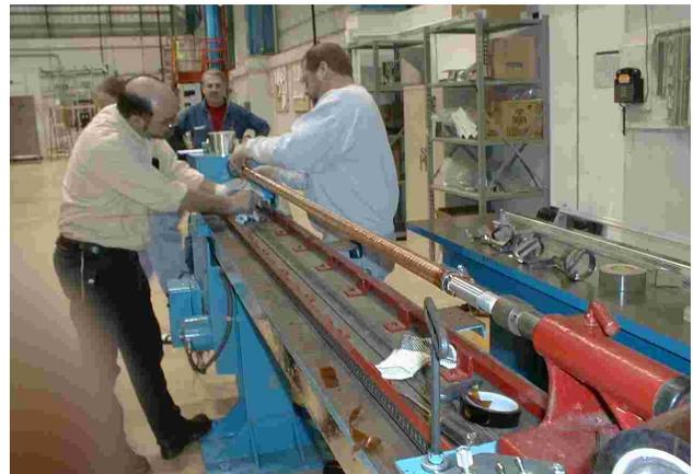
Fig. 10 – Spiral-wrapping of copper tape on prototype transmission line lengths using the wrapping machine used for Tevatron and Recycler beam pipes. The conductor design and swaging operation have been chosen to allow in-house production of 70m lengths.
