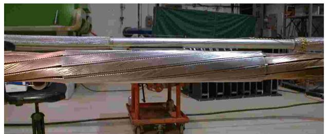
Fig. 6 – Completed splice for the conductor test loop. After soldering, the conductor is wrapped in copper tape to allow clamshell welding of the helium pipe over the splice. The vacuum jacket is made up with telescoping sections over the splice region.
