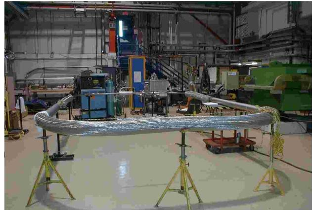
Fig. 9 – 100kA conductor test loop nearing completion. Dewar-based cryogenic system in background and drive transformer at right. The test loop contains a 4m replaceable test section of transmission line
