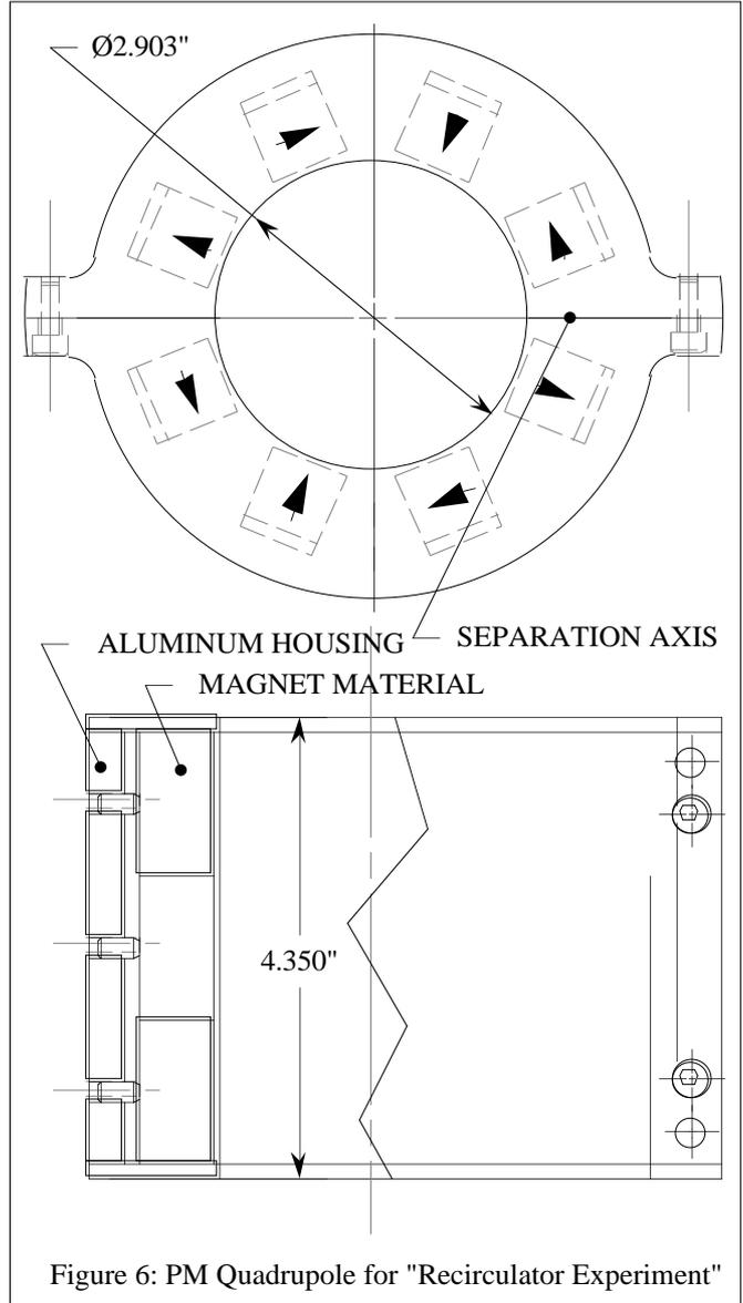
one orientation. The design for these PMQ's is shown in Figure 6. This design allows the quadrupole magnets to be split so that they may be easily be installed over the vacuum chamber.
