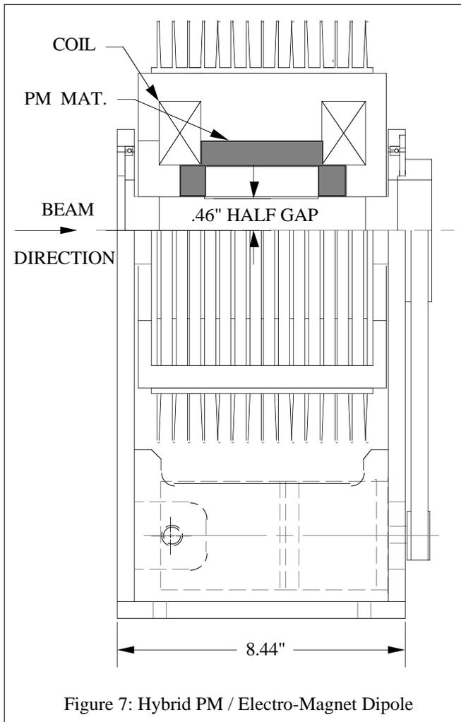
Figure 7: Hybrid PM / Electro-Magnet Dipole
