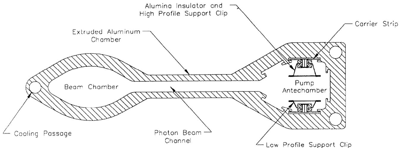
Figure 1. Storage Ring Vacuum Chamber Cross Section.
