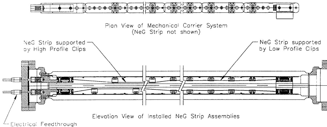
Figure 2. Typical Installation of NeG Assembly.
