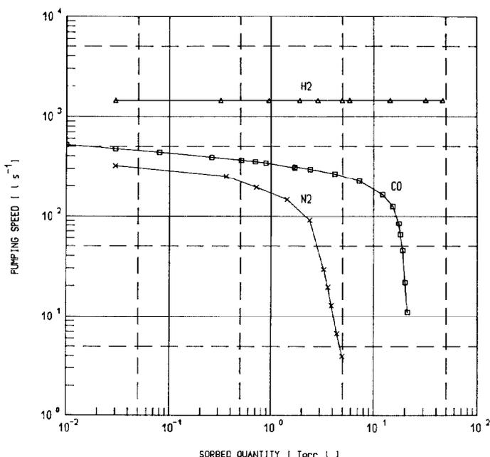
FIG.2 room temperature sorption curves (CO, N<sub>2</sub> and H<sub>2</sub>) for the HCGP prototype
