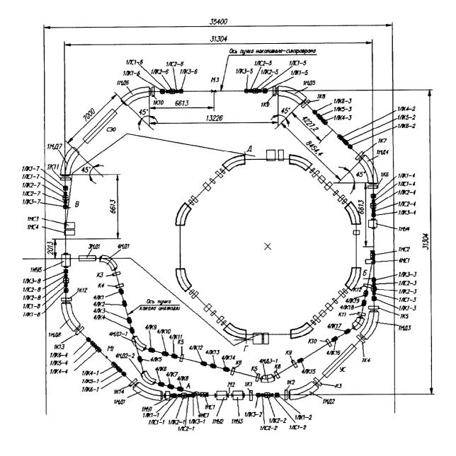
Fig.1. The INR (Kiev) Storage-Accelerating Complex
