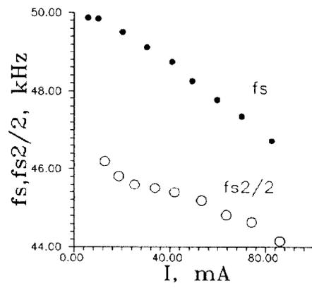
Figure 4: Current dependence synchrotron frequencies at 600 MeV.
