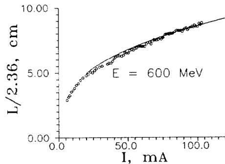
Figure 5: Calculated current dependence bunch length.
