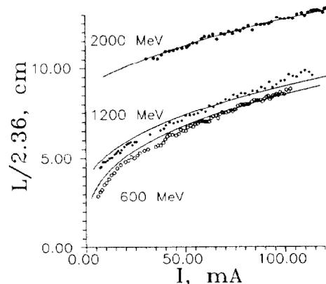
Figure 1: Bunch length versus current ( $L$  - halfwidth bunch length,  $s = L/2.56$ ).
