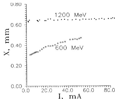
Figure 2: Current dependence bunch horizontal transverse size.
