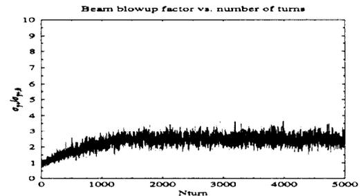
Figure 3: Beam blowup for the  $e^+$  beam during 5000 turns for parameters in Table 2.
