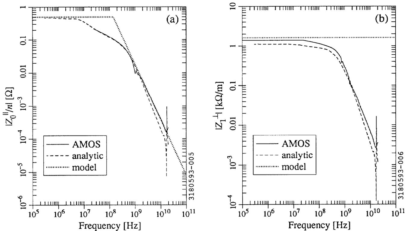
Figure 4. Predicted (a)  $|Z_0^{\parallel}/n|$  and (b)  $|Z_1^{\perp}|$  for a full-size TT2-111V load, along with model values used for ZAP.
