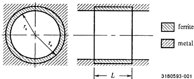
Figure 1. Load geometry. For a full-size load,  $L = 150$  mm,  $r_x = 118.4$  mm, and  $r_o = 121.6$  mm.
