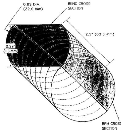
Fig. 3. The new bend-to-quad transition.
