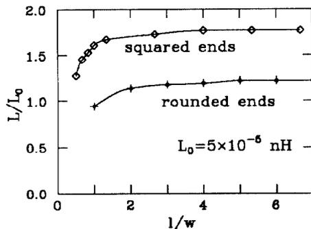
Fig. 4. The inductance of a slot;  $w = 1.5$  mm.
